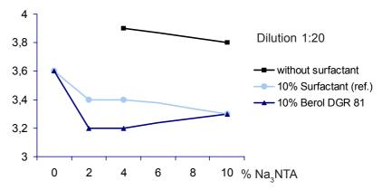
Tests have shown that 4%  ${\rm Na_3NTA}$  and 10% Berol DGR 81, diluted 1:20, is enough for obtaining a good result at high pressure cleaning.
