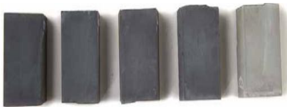
Left to right: Carbocolor loaded at 6%, 4%, 3%, 2%, and a reference blank.
